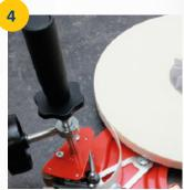
As an option, you can use the edge guide roller to aid in accurate application of UHB Tape. This is an option and not essential for effective use of the UHB-001 applicator.
