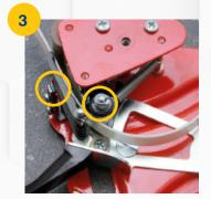
Thread the UHB Tape between pressure roller and trimmer unit, hand dispenser is ready to use. There is a width guide O ring that must be slid to match the tape width to stop tracking.
