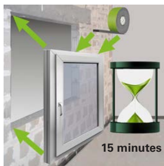
Figure 4: Install the window within 15 minutes.
