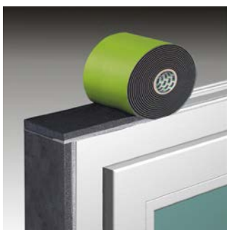
Figure 3: Affix TP652 to the frame - side with the grey step inwards. Allow projection on the corners.
