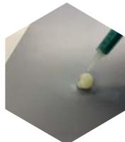
**Step 4:** Apply a blob of adhesive to the substrate. Ideal size would be same diameter as locator foot at approx. 2-3mm high.
