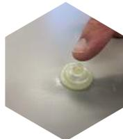
**Step 5:** Place the locator into the adhesive. Do not force it flat to the substrate. Just move around gently so that the adhesive comes out of the edge and bonds to the outer diameter of the foot. You should be left with approx. 0.5mm-1mm thick adhesive between foot and substrate.
