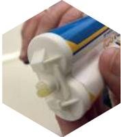
**Step 3:** Place cartridge into gun and remove cap. Gently squeeze trigger until adhesive appears in left and right outlet. This is to burp the cartridge. Fix nozzle in place and dispense a small amount into a waste container to ensure you have a perfect mix.
