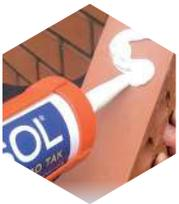
**Step 2:** Apply the SIGNBONDER to the sign or substrate being bonded to the wall in beads not blobs. Blobs will take a lot longer to cure and run the risk of not fully curing in the centre of the adhesive. Position onto the surface where required. You will be able to move the sign around to position. Press sign in place, but not too much as you need to leave about 1mm of adhesive between sign and wall.
