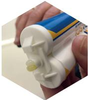
**Step 3:** Place cartridge into gun and remove cap. Gently squeeze trigger until adhesive appears in left and right outlet. This is to burp the cartridge. Fix nozzle in place and dispense a small amount into a waste container to ensure you have a perfect mix.
