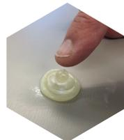
**Step 5:** Place the locator into the adhesive. Do not force it flat to the substrate. Just move around gently so that the adhesive come out of the edge and bonds to the outer diameter of the foot. You should be left with approx. 0.5mm-1mm thick adhesive between foot and substrate.
